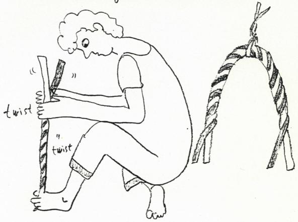
Take center of hando and twist a short piece of rope (10") around it.
